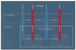
Figure 5 - Hot aisle containment
